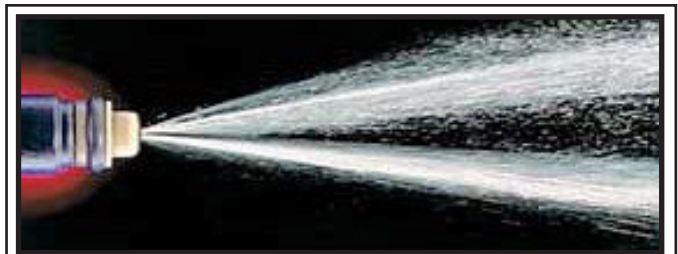
Poor Spray Pattern caused by carbon build-up in Port Fuel Injector prior to DZL-LENE XL/10 treatment.
